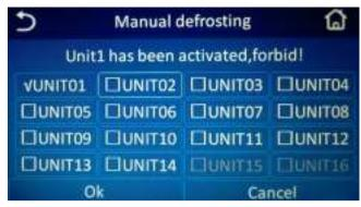
(e) When this function has been enabled for five minutes, however the unit fails to perform defrosting.
