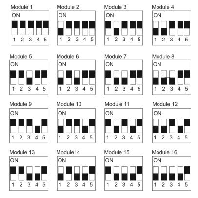
Note: the black block represents where the projecting lever of the DIP switch is.
