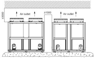
Note: Shock pads (prepared by clients)should be fit to unit bases and fixed with screws to the ground or roofs.
