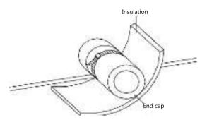
Insulation should be thickened at humid areas. You could follow the procedures of insulating refrigerant pipes.
