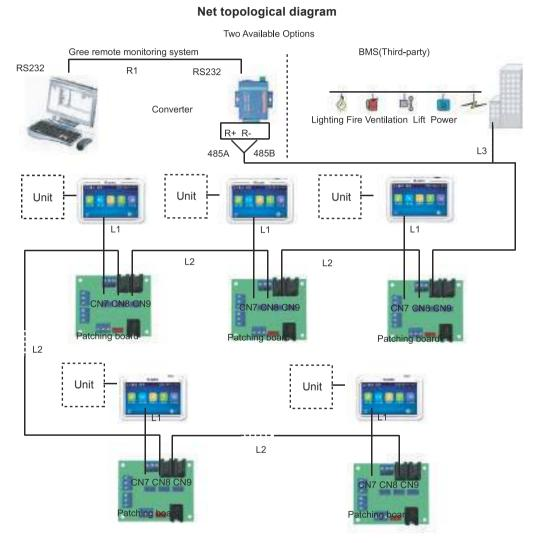
Note: the system as shown in the figure above consists of 1~16 single units depending on the actual demand of the project.
