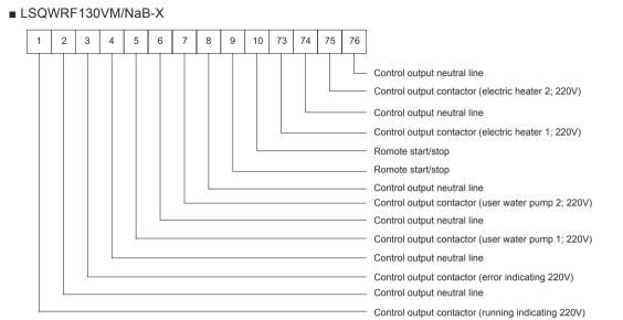
Note: the output control lines of the AC contactors for the running indicator, water pump 1, water pump 2, auxiliary electric heater 1, auxiliary electric heater 2 can be wired to the corresponding wiring board of any one unit, while those for the error indicator and external passive contact switch should be wired to the corresponding wiring board of all units as shown in the figure below.
