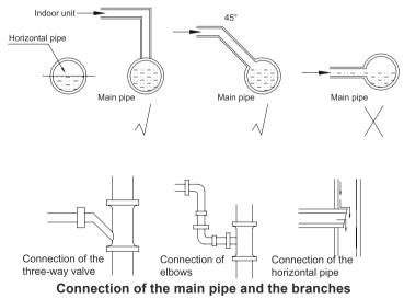
When the three-way valve is used for the condensate pipe, its straight two connectors should be kept at the same level as shown in the figure below.
