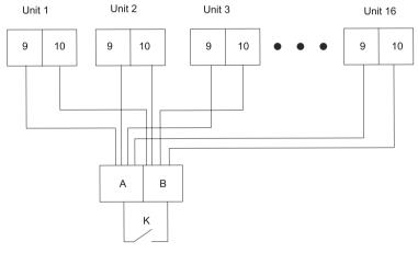
When external passive contact switch is available for multiple units, the wiring board 9 and 10 of each unit should be wired to the dry contact A and B.
