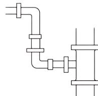
Connection of drain elbow
