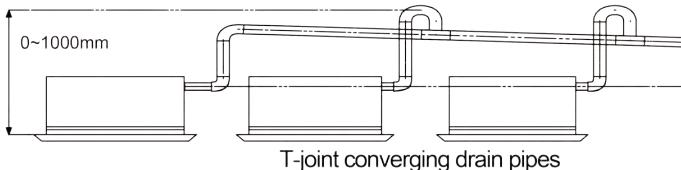
T-joint converging drain pipes
