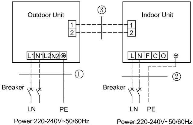
2). The Power Supply for indoor unit from outdoor unit:
