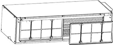
Press the return air inlet filter downward against the guide groove sponge and take it off along the arrow direction. There are two return air inlet filters.
