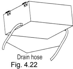
As the inside of the unit is in the negative pressure status, it is required to set backwater elbow. The requirements is:
