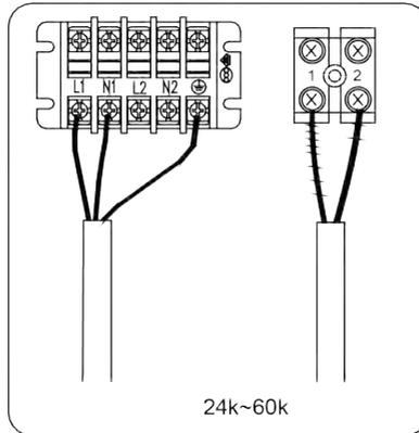
2). The Power Supply for indoor unit from outdoor unit:
