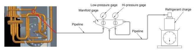
Refrigerant charge is determined through stringent tests, as excess or shortage of refrigerant would cause the compressor to run improperly. Thus, the refrigerant charge shall be consistent with that specified on the nameplate. If refrigerant charge is indeed insufficient, follow the steps below for adding.
