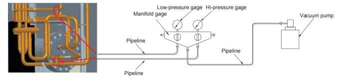
Step 3: Open the valves at both the high-pressure and low-pressure sides and then start the vacuum pump until the gage reading is below -1bar. After that, let the vacuum pump lasts for another 0.5~1.0 hour.
