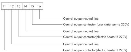
Note:The output control lines of the auxiliary electric heater 1, auxiliary electric heater 2 and the water pump AC contactor are allowed to the terminal boards 11/12/13/14/15/16 of any module.
