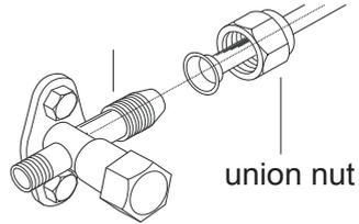
4. Tighten the union nut with torque wrench by referring to the sheet below.
