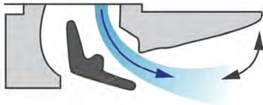
Horizontal air supply in cooling
