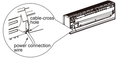
3. Remove the wire clip; connect the power connection wire to the wiring terminal according to the color; tighten the screw and then fix the power connection wire with wire clip.
