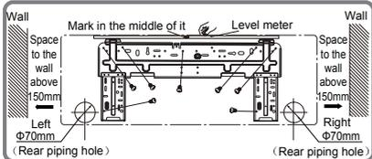
2. Open a piping hole with the diameter of  $\Phi 55$  or  $\Phi 70$  on the selected outlet pipe position. In order to drain smoothly, slant the piping hole on the wall slightly downward to the outdoor side with the gradient of  $5-10^\circ$ .
